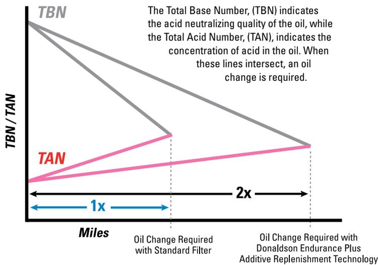
\* Field test results conducted on Class 8 trucks powered by Detroit Diesel Series 60 engines and SAE 15W-40 CI-4 oil.
